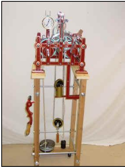
Gravity train remontoire: Endless chain design. Robert Robin, France, 1772; based on earlier maintaining power design by Christiaan Huygens, Holland, 1658. (center diagram).
