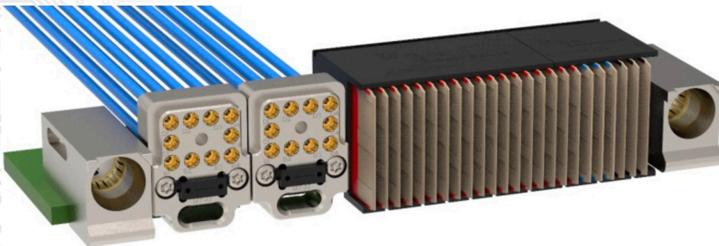
Figure 2. Rear view of 3U OpenVPX Module with two VITA 67.3D backplane connectors, each with 10 coaxial RF signals and 24 optical lanes. Courtesy TE Connectivity
