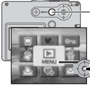
To delete a displayed image, use the main playback menu. Press the menu button to display the main menu on the LCD monitor.
