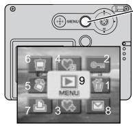
With playback-mode activated, pressing the menu button displays the main playback menu. The following nine options are available:
