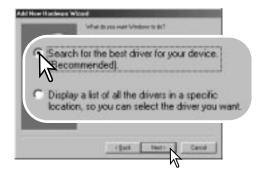
Choose to specify the location of the driver. The browse window can be used to indicate the driver location. The driver should be located in the CD-ROM drive at :\Win98\USB. When the location is shown in the window, click "Next."
