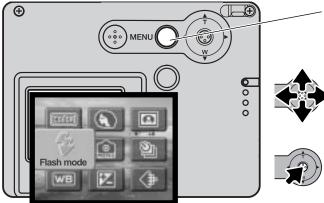
To activate the main menu of the recording mode, press the menu button.
