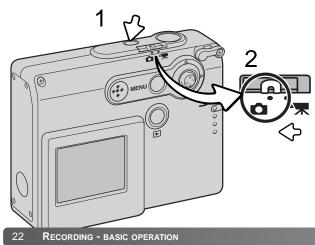
Turn the camera on by pressing the main switch near the shutter-release button (1).
