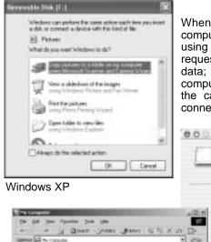
When the camera is properly connected to the computer, a drive icon, or volume, will appear. When using Windows XP or Mac OS X, a window will open requesting instructions on what to do with the image data; follow the directions in the window. If the computer does not recognize the camera, disconnect the camera and restart the computer. Repeat the connection procedure above.
