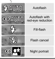
**Autoflash -** the flash fires automatically in lowlight and backlit conditions.
