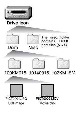
Files and folders on the memory card can be deleted using the computer. Never format the memory card from the computer; always use the camera to format the card. Only files recorded by the camera should be stored on the memory card. Image file names begin with "PICT" followed by a four-digit file number and a jpg or mov extension. The jpg extension indicates a still image, and the mov extension, a movie clip.
