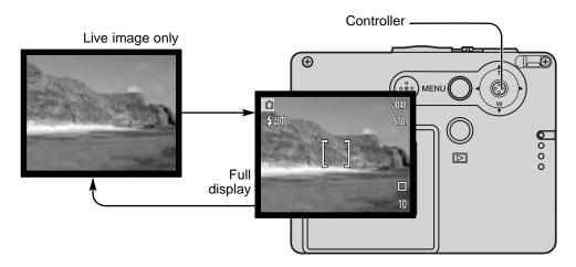
The battery-condition, date-imprinting, and flash-charging indicators can appear on the live image only display. When auto reset is active, the LCD monitor is reset to the full display when the camera is turned off.
