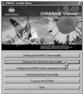
Before connecting the camera to the computer, place the DiMAGE Viewer CD-ROM in the CD-ROM drive. The DiMAGE installer menu should automatically activate. To automatically install the Windows 98 USB driver, click on the starting-upthe-USB-device-driver-installer button. A window will appear to confirm that the driver should be installed; click "OK" to continue.
