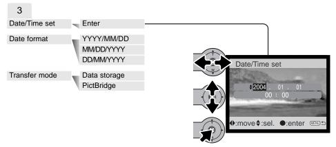
On the date/time setting screen, move the controller left and right to select the year, month, day, hour, or minute. Move the controller up and down to change the value. Press the controller to set the calendar and clock.
