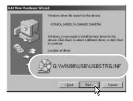
The add new hardware wizard will confirm the location of the driver. One of three drivers may be located: MNLVENUM.inf, USBPDR.inf, or USBSTRG.inf. The letter designating the CD-ROM drive will vary between computers. Click "Next" to install the driver in the system.
