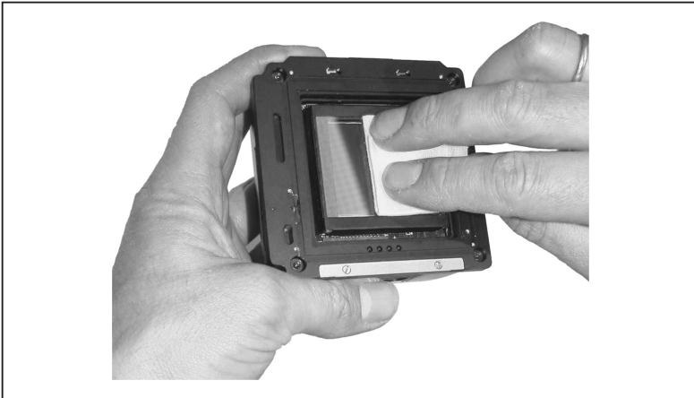
Figure 10: Cleaning the Infrared Filter
