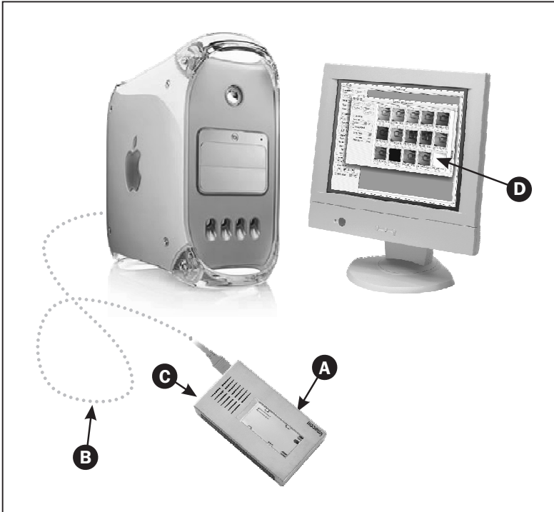
Figure 6: Connecting the Image Bank to the computer
