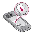
3 Insert the battery into place by aligning the gold contacts on the phone and the battery.
